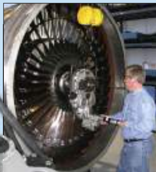
Model 8300 being used with 8202A air driven multiplier
